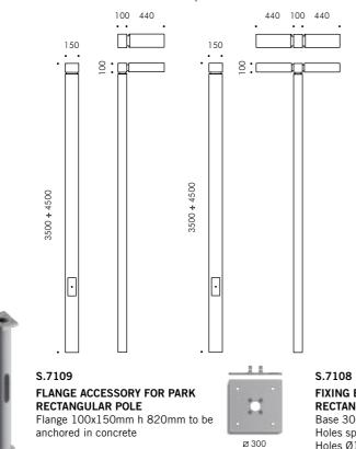
FIXING BASE FOR PARK RECTANGULAR POLE Base 300x300mm Holes spacing 200x200mm Holes Ø18mm for M16 bolts
