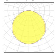
LED CCT 3783 K Lamp type Nominal lamp power 0.48 W CRI 80 Total flux LOR 100% 36 lm Luminous efficacy 75 lm/W Total power 0.48 W
