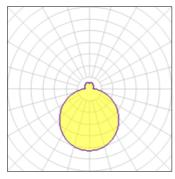
Lamp type LED Nominal lamp power 21 W Total flux 1900 lm Luminous efficacy 90 lm/W
