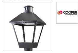
Aluminum housing, top, and base, Greater than 98% life at 60,000 hours ( $40^{\circ}$ C) (LED), Up to 140 lumens per watt, Lumen packages ranging from 2,000 – 11,000 lumens, Self-aligning pole-top fitter fits 2-3/8" and 3" O.D. tenons, Optional NEMA photocontrol receptacle, Five-year warranty (LED)
