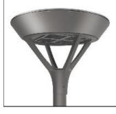
Die-cast aluminum housing and door, Lumens packages ranging from 3,000 - 29,000 lumens, Choice of 13 high-efficiency, patented AccuLED Optics™, Base casting slip fits over a standard 3" O.D. tenon, Wall, single and dual-mount configurations available, 10kV/10vkA surge protection standard, LED fixture features a five-year warranty
