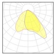
1 x LED Nominal lamp power 72 W LOR 81% Lamp flux 8400 lm Total flux 6812 lm Luminous efficacy 117 lm/W Total power 80 W CCT 2700 K CRI 80
