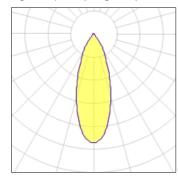
Lamp typeLEDCCTNominal lamp power45 WCRITotal flux3600 lmLORLuminous efficacy80 lm/WTotal power
