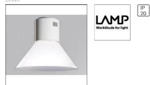
Suspended downlight model STORMBELL 3000 NW WFL WH/WH., LAMP brand. Made of shiny white extruded and injected aluminum body with polycarbonate opal ring. Model for COB with neutral white color temperature and control gear included on white decorative rose. Wide Flood aluminum reflector. Insulation class I.
