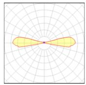
Lamp type LED CCT 6000 K CRI Nominal lamp power 6.4 W 70 Total flux 60 lm LOR 100% Luminous efficacy 9 lm/W ULOR 65% Total power 6.4 W
