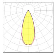
Lamp type LED CCT 3000 K Nominal lamp power 6 W CRI 80 Total flux LOR 100% 300 lm Luminous efficacy 50 lm/W Total power 6 W
