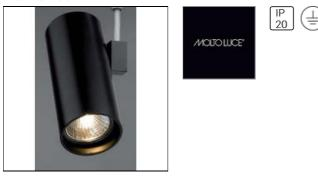
Shooter 1, Ceiling Spotlight, its simple and compact design is ideal for accent lighting; made of high-quality, die-cast aluminum; black powder coated finish; lamp replace without tools by "Slide Change"; 1x max.50W QPAR16 GU10, 230V; 340 ° rotation and 90 ° tilt, IP 20;
