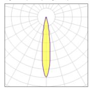
LED CCT 3000 K Lamp type Nominal lamp power 4 W CRI 80 Total flux LOR 100% 158 lm Luminous efficacy 40 lm/W Total power 4 W
