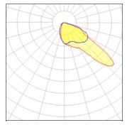
Lamp typeLEDCCTNominal lamp power104 WCRITotal flux12376 lmLORLuminous efficacy119 lm/WTotal power
