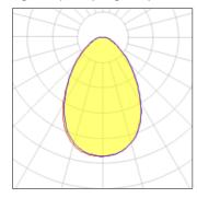
Lamp typeLEDCCTNominal lamp power12.5 WCRITotal flux1220 lmLORLuminous efficacy98 lm/WTotal power
