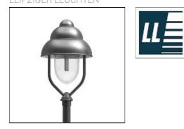
For medium and high light requirements, mounting height 3.80 m. - Impact-resistant clear polycarbonate attachment, UV-stabilized, -Aluminium luminaire body, inside finished in white paint, outside painted in colour - Aluminium unit carrier, painted white - Adapter jack connection -Available in any RAL or DB colour without surcharge - Scope of supply includes fork bracket,post dia. 76 mm (for 3,80 m mounting height) and ornamental ring, painted
