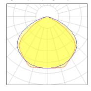
Lamp type LED CCT 5181 K Nominal lamp power 411 W CRI 86 Total flux LOR 100% 52029 lm Luminous efficacy 127 lm/W Total power 411 W
