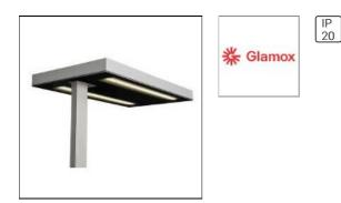
Light source: LED Lumen out: 8825 CRI: 80 Colour temperature: 4000 Total effect: 82 Lumen per watt: 108 Optic: BL Driver: DALI;HF Main body material: Acrylic/Aluminium
