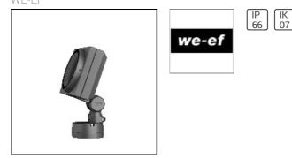
IP66, Class I. IK07. Marine-grade, die-cast aluminium alloy. 5CE superior corrosion protection including PCS hardware. Silicone CCG® Controlled Compression Gasket. Safety glass lens. Integral EC electronic converter in thermally separated compartment. CAD-optimised optics for superior illumination and glare control. OLC® One LED Concept. Factory installed LED circuit board. The luminaire is factory- sealed and does not need to be opened during the installation.
