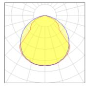
LED CCT 4000 K Lamp type Nominal lamp power 33 W CRI 80 Total flux 4454 lm LOR 100% Luminous efficacy 135 lm/W Total power 33 W
