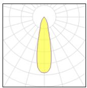
Lamp type LED CCT 2700 K Nominal lamp power 21 W CRI 90 Total flux 2260 lm LOR 100% Luminous efficacy 108 lm/W Total power 21 W
