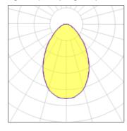
Lamp type LED CCT 3000 K Nominal lamp power 7.48 W CRI 80 Total flux 563 lm LOR 100% Luminous efficacy 75 lm/W Total power 7.48 W
