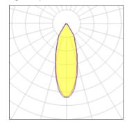
1 x LED Nominal lamp power Lamp flux 1750 lm Luminous efficacy 77 lm/W 3000 K CRI
