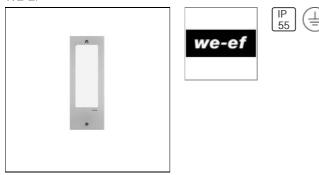
IP55, Class I. IK10. Marine-grade, die-cast aluminium alloy. 5CE superior corrosion protection including PCS hardware. Silicone rubber gasket. Polycarbonate main lens. Two cable entries. Factory installed LED circuit board. Integral EC electronic converter. A pre-installation blockout is available and recommended for mounting in concrete walls.
