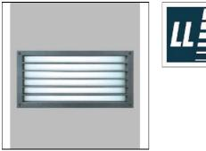
Luminaire constructed for the variable installation in walls or steps, in order to illuminate ways and staircases. - Impact-resistant opal polycarbonate cube, UV-stabilized - luminaire body and unit carrier, made of corrosion-resistant cast aluminium, availablel painted in any RAL or DB colour without surcharge - Luminaire body completely detachable for lamp replacement, opens with tool - with cable joint box suitable for cables 5 x 2,5 mm2 - suitable for incoming cables
