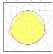
Lamp typeLEDCCTNominal lamp power95 WCRITotal flux13300 lmLORLuminous efficacy140 lm/WTotal power
