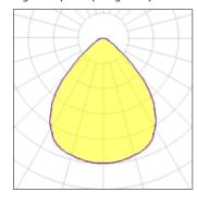
Lamp type LED CCT 3000 K Nominal lamp power 37.92 W CRI 81 Total flux 3800 lm LOR 100% Luminous efficacy 100 lm/W Total power 37.92 W
