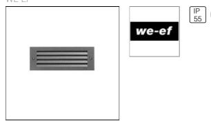
IP55, Class I. Marine-grade die-cast aluminium alloy. 5CE superior corrosion protection including PCS hardware. Silicone rubber gasket. Polycarbonate main lens. Two cable entries. A pre-installation blockout is available and recommended for mounting in concrete walls. To be ordered separately.
