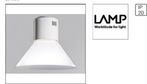
Suspended downlight model STORMBELL 5000 WW FL WH/WH., LAMP brand. Made of shiny white extruded and injected aluminum body with polycarbonate opal ring. Model for COB with warm white color temperature and control gear included on white decorative rose. Flood aluminum reflector. Insulation class I.
