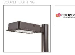
One-piece, die-cast aluminum housing can be pole or wall-mounted, Optical design creates consistent distribution and scalability, Choice of 12 high-efficiency, patented AccuLED Optics<sup>™</sup>, Standard in 4000K (+/- 275K) CCT and nominal 70 CRI, Suitable for operation in -40°C to 40°C ambient environments, 120-277V 50/60Hz, 347V 60Hz or 480V 60Hz operation, Proprietary circuit module withstands 10kV of transient line surge, Optional battery pack and bi-level switching, Five-year warranty
