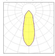
Lamp type LED CCT 3000 K Nominal lamp power 7.5 W CRI 80 Total flux 470 lm LOR 100% Luminous efficacy 63 lm/W Total power 7.5 W
