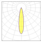
CCT 3000 K Lamp type LED Nominal lamp power 2.75 W CRI 90 Total flux 201 lm LOR 100% Luminous efficacy 73 lm/W Total power 2.75 W
