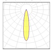
LED CCT 3000 K Lamp type Nominal lamp power 2.75 W CRI 90 Total flux 201 lm LOR 100% 73 lm/W 2.75 W Luminous efficacy Total power
