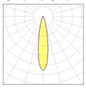
CCT Lamp type LED 3000 K Nominal lamp power 2.75 W CRI 90 Total flux 201 lm LOR 100% Luminous efficacy 73 lm/W Total power 2.75 W
