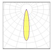
3000 K Lamp type LED CCT Nominal lamp power 2.75 W CRI 90 Total flux 201 lm LOR 100% Luminous efficacy 73 lm/W Total power 2.75 W
