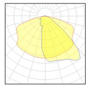
1 x LED Nominal lamp power 51 W LOR 73% Lamp flux 6450 lm Total flux 4683 lm Luminous efficacy 126 lm/W Total power 57 W CCT 3000 K CRI 80
