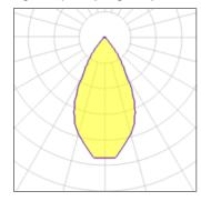
LED CCT 4000 K Lamp type Nominal lamp power 8 W CRI 80 Total flux 546 lm LOR 100% Luminous efficacy 68 lm/W Total power 8 W
