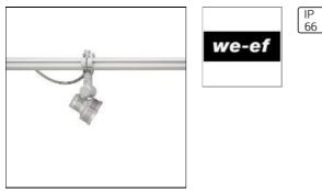
IP66. Marine-grade die-cast aluminium alloy. 5CE superior corrosion protection including PCS hardware. Silicone rubber gaskets. Safety glass lens. Anodised aluminium reflector.Including 0,4 m of flexible cable enclosed in stainless conduit, in-line connector and mounting clamp for installation to RAIL66 mounting system.
