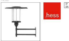
Round luminaire canopy made of aluminium, plain coloured. Support elements made of stainless steel. Cylindrical luminaire enclosure made of PMMA. Round luminaire body made of aluminium. 10.45700.0V002 MADRID 600 Wall bracket MADRID 600/600-2 Made of galvanised steel Overhanging 500 mm Colour: DB 703 or all RAL- (classic- single shades), Hess-DB and Hess-Glimmer-colours. RAL pearl-mica-metallic-shades on request.
