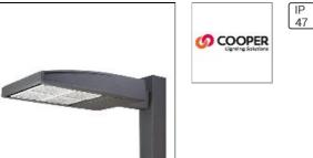
Choice of 16 high-efficiency, patented AccuLED Optics™, Lumen packages range from 4,200 - 80,800 (34W - 640W), Available in 2200K, 2700K, 3000K, 3500K, 4000K, 5000K or 5700K CCT, -40°C to 40°C operating range, optional 50°C high ambient, 120-277V 50/60Hz, 347V 60Hz or 480V 60Hz operation, IP66 rated housing and light square, 3G vibration rated, Pole, mast-arm or wall-mounted configurations, Fiveyear warranty
