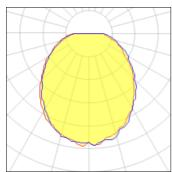
Lamp typeCCT3000 KNominal lamp power17 WCRI80Total flux1624 lmLOR100%Luminous efficacy96 lm/WTotal power17 W
