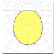
Lamp typeCCT3000 KNominal lamp power17 WCRI80Total flux1624 lmLOR100%Luminous efficacy96 lm/WTotal power17 W
