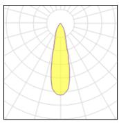
Lamp type LED CCT 2700 K Nominal lamp power 29.2 W CRI 90 Total flux 3090 lm LOR 100% Luminous efficacy 106 lm/W Total power 29.2 W
