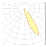
LED CCT 2700 K Lamp type Nominal lamp power 8 W CRI 80 Total flux LOR 100% 428 lm Luminous efficacy 54 lm/W Total power 8 W
