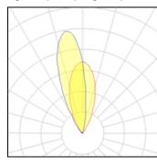
Lamp typeLEDNominal lamp power2.9 WTotal flux179 lmLuminous efficacy62 lm/W
