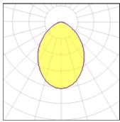
1 x LED Nominal lamp power 49.7 W LOR Lamp flux 5107 lm Total flux
