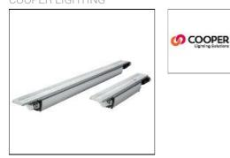
Cove lighting fixture with integral driver, Up to 1500 lm/ft (3 light level options at 500, 1000 and 1500 lm/ft), IP66 rated for continuity of lighting from interior to exterior spaces, 1% dimming, 0-10V (1% - 100%), 90 CRI standard, Up to 130 lm/W, Up to 300 ft run from a single power drop, Self-closing end cap + quick connects for easy error-free installation, Self-aligning brackets with 15 and 30 degree mounting angle options
