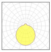
Lamp type LED CCT 3000 K Nominal lamp power 17 W CRI 80 Total flux 2020 lm LOR 100% Luminous efficacy 119 lm/W ULOR 17% Total power 17 W
