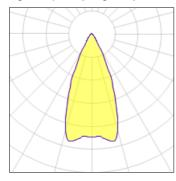
Lamp type LED CCT 3000 K Nominal lamp power 30 W CRI 90 Total flux LOR 100% 2250 lm Luminous efficacy 75 lm/W Total power 30 W
