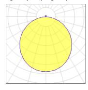
Lamp type Nominal lamp power Total flux Luminous efficacy LED 24 W 2530 lm 105 lm/W CCT
