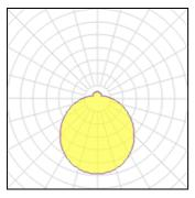
Lamp type LED CCT 3000 K Nominal lamp power 28 W CRI 80 Total flux 3470 lm LOR 100% Luminous efficacy 124 lm/W ULOR 15% Total power 28 W
