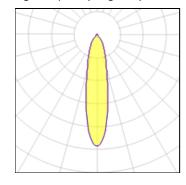
Lamp type Nominal lamp power Total flux Luminous efficacy LED 27 W 2150 lm 80 lm/W CCT
