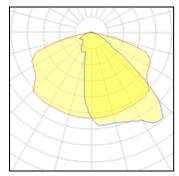
1 x LED Nominal lamp power 72 W LOR 73% Lamp flux 8400 lm Total flux 6099 lm Luminous efficacy 117 lm/W Total power 80 W CCT 2700 K CRI 80
