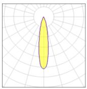
CCT 2700 K Lamp type LED Nominal lamp power 2.75 W CRI 90 Total flux 186 lm LOR 100% Luminous efficacy 68 lm/W Total power 2.75 W
