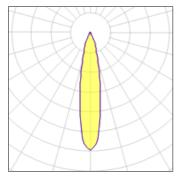
CCT 4000 K Lamp type LED Nominal lamp power 2.75 W CRI 90 Total flux 215 lm LOR 100% Luminous efficacy 78 lm/W Total power 2.75 W
