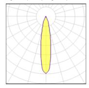
LED CCT 4000 K Lamp type Nominal lamp power 2.75 W CRI 90 Total flux 215 lm LOR 100% 78 lm/W 2.75 W Luminous efficacy Total power
